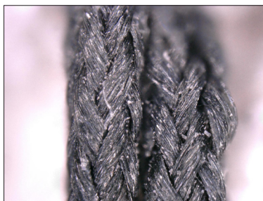
Fig. 13a: Black braided silk sutures magnified 200-fold with Keyence VHX-5000 microscope shows the texture of wax and silicone. Image: Nicole Ong Yui Mei
