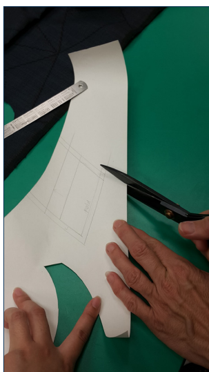
Fig 21.2: The desired pocket size is drawn and cut. The parts are sewn to the lining of the outer fabric and ironed to flatten. Mihaleva checks that the flap is aligned to the pocket. Images: Ong Xin Hong
